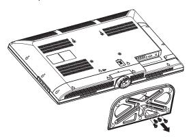
**3** Remove the four screws that secure the stand column, then remove the column.
